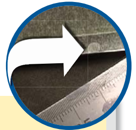
Typical weld margin contamination
