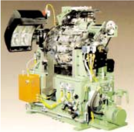
Reynolds RT-6 Light Tester fitted with the ULTP up-grade
