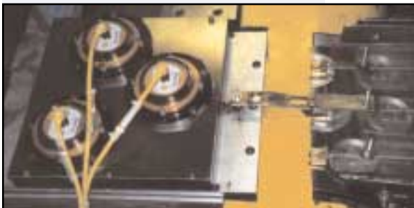
The ELTP Light Detectors are Mounted at the Discharge of the End Conversion Press
