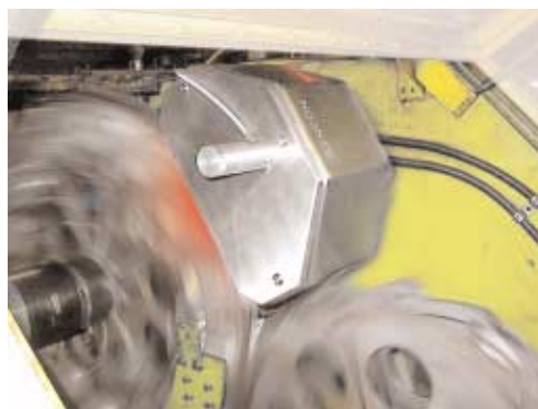
label inspector mounted inside an Alcoa LT16 Light Tester
